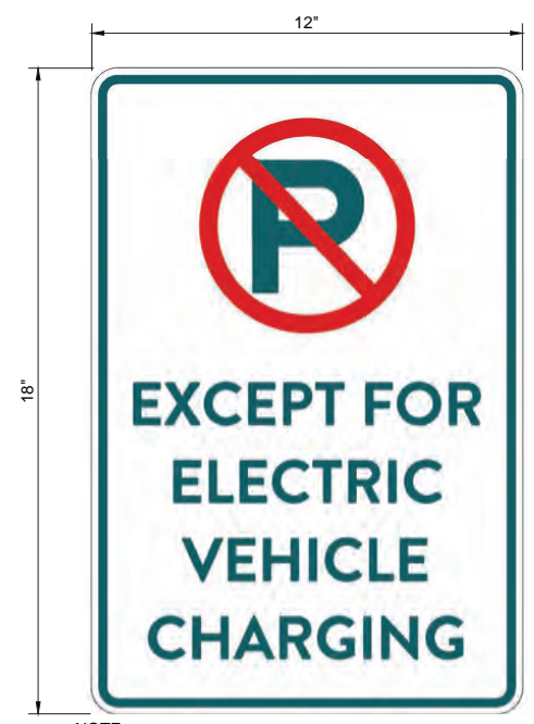
3 ACCESS AISLE SIGN C5.02 NOT TO SCALE
